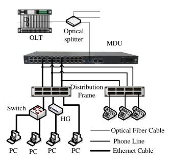
Figure 3-1 Cable connection
